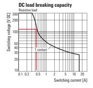
The curve shows a maximum switching current of approx. 0.45 A with resistive load. This must now be set in relation to the rated current of the relay (16 A) from the data sheet and the value for a DC13 load from the table.
